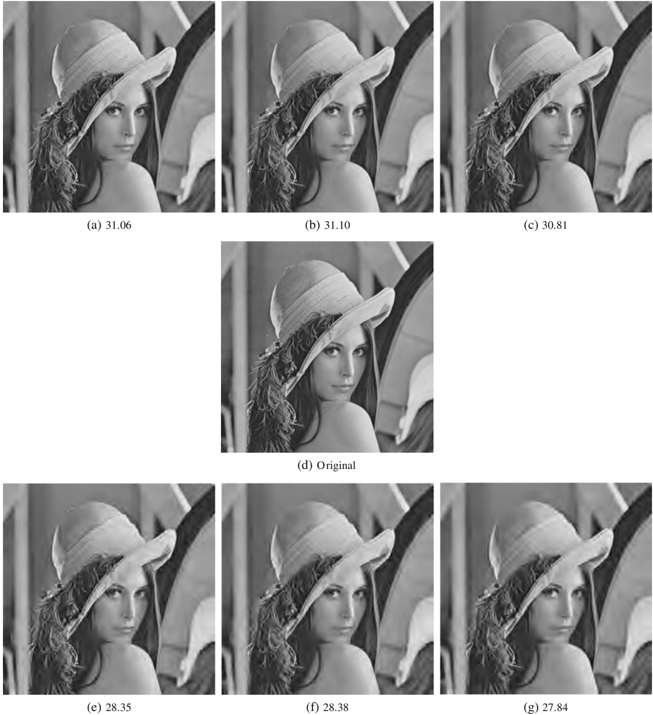
Figure 11 Lena compressed at 0.125 bpp a LTW_RCi_2%, b SPIHT, c JPEG2000 and Lena compressed at 0.0625 bpp e LTW_RCi_2%, f SPIHT, g JPEG2000.
