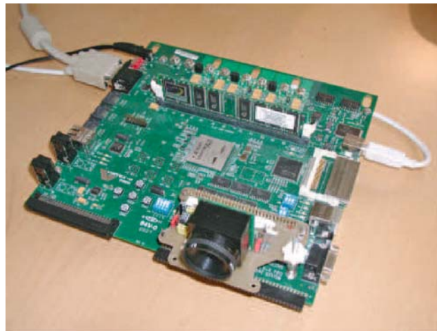
Figure 13. Xilinx XUP Virtex-II Pro FPGA development board with attached sensor.
