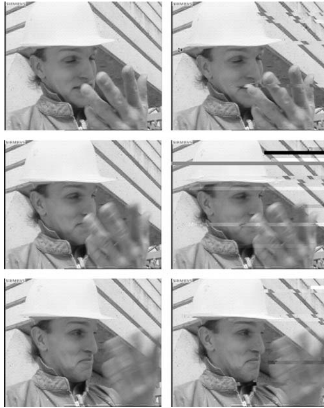
Figure 12. Comparisons of image quality between the watermarked frames (left column) and the received frames (right column) over the channels with BER = 10^{-4} .
