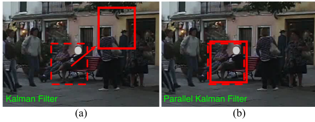
Fig. 6 Illustration of the escape problem. a, b Display the predicted trajectories of the same bounding box by KF and PKF, respectively, after the tracked person gets lost. The red dashed box represents the box at the beginning of the lost trajectory; the red solid box represents the box after 15 consecutive prediction phases of KF or PKF. The box predicted by the KF escapes in the direction of the velocity with noise, while the PKF suppresses the noise and keeps the box around the dashed box so that the person can be retraced (Color figure online)
