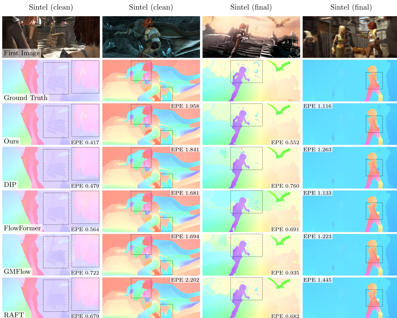
Fig. 9 Visual comparison to other methods from the literature for the MPI Sintel benchmark. First row. Four exemplary frames. Other rows. Computed flow fields. Note the differences in the marked locations. Best viewed electronically
