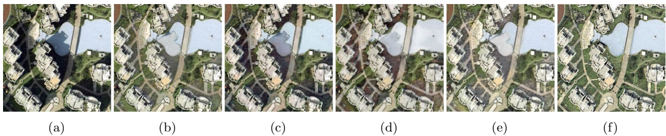
Fig. 22 Comparison with the state-of-the-art methods on a remote sensing shadow image (a). b–e are results of G2R-ShadowNet (Liu et al., 2021), Auto-Exposure (Fu et al., 2021), DC-ShadowNet (Jin et al., 2021), and wSP+M-Net (Le & Samaras, 2021). f Our result
