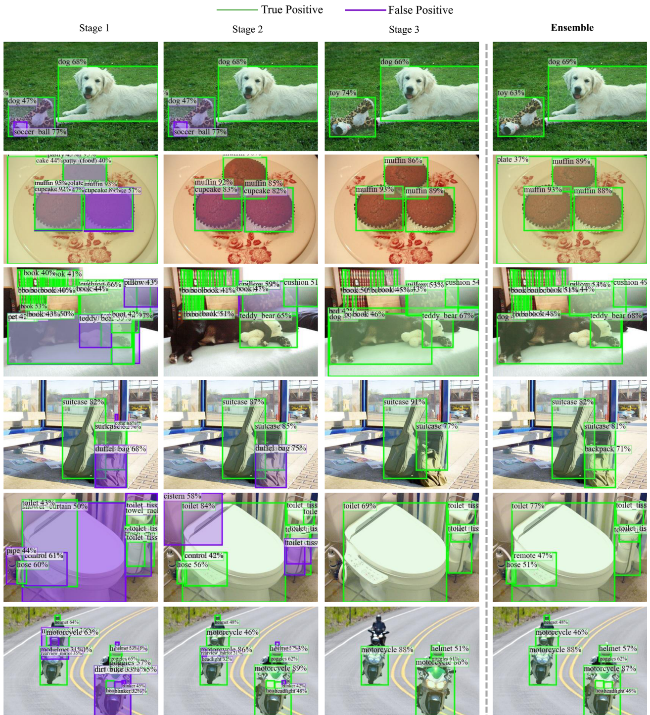
Fig. 4 The pseudo labels generated on the LVIS training dataset under the semi-supervised object detection setting (SSOD) setting. The green color refers to the true-positive predicted results; purple color refers to false-positive detection results (Zoom in for best view) (Color figure online)
