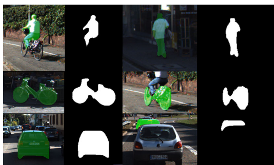
Fig. 3 Intra-class variation of detected instances, where we show examples variations of the pose of a detected person (top row), missing bike handlebar (middle row) and occlusion effects on a detected car (bottom row)
