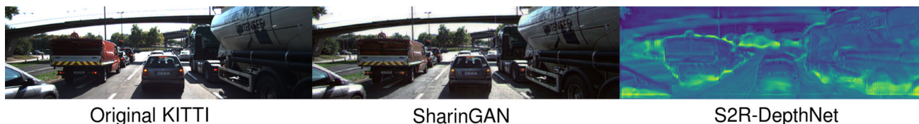
Fig. 12 Transfer of KITTI images to the intermediate shared domain employed by SharinGAN (PNVR et al., 2020) and S2R-DepthNet (Chen et al., 2021). The original single-channel S2R-DepthNet images are mapped to RGB using a colormap and logarithmic mapping
