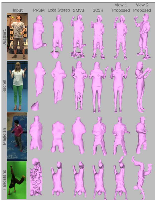
Fig. 7 Reconstruction evaluation against existing methods. Two different views of 3D model are shown for proposed method
