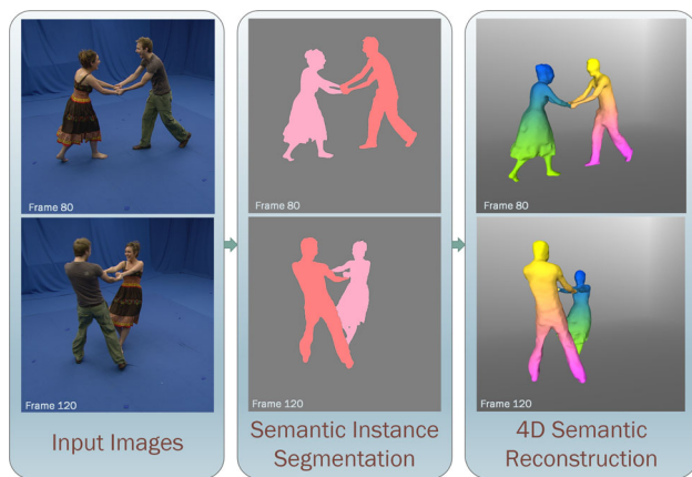
Fig. 1 Joint 4D semantic instance segmentation and reconstruction exploiting 3D human-pose of interacting people in dynamic scenes. Shades of pink in segmentation represents instances of people. Colour assigned to reconstruction of frame 80 is reliably propagated to frame 120 using proposed temporal coherence (Color figure online)
