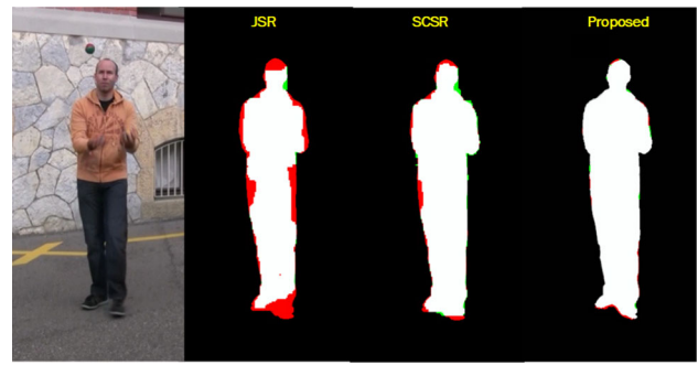
Fig. 11 Ground-truth semantic segmentation comparison against state-of-the-art methods JSR and SCSR
