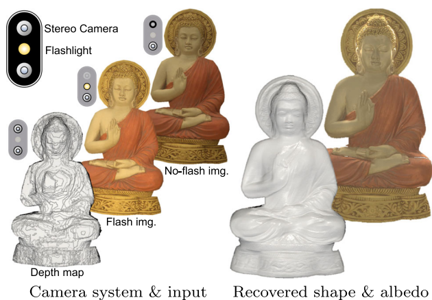
Fig. 1 Our setup uses a stereo camera and a flashlight, which is common in modern smartphones, e.g. , the iPhone X from 2017. We capture a stereo image pair to infer a rough depth map and a flash/no-flash image pair to recover shape details and surface albedo
