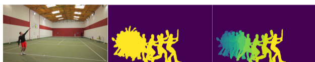
Fig. 6 Examples of an input video frame, the corresponding motion energy image and motion history image computed by Bobick and Davis (2001)
