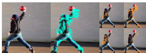
Fig. 7 Examples of the original frame, optical flow, and the flow field in four channels computed by Efros et al. (2003)
