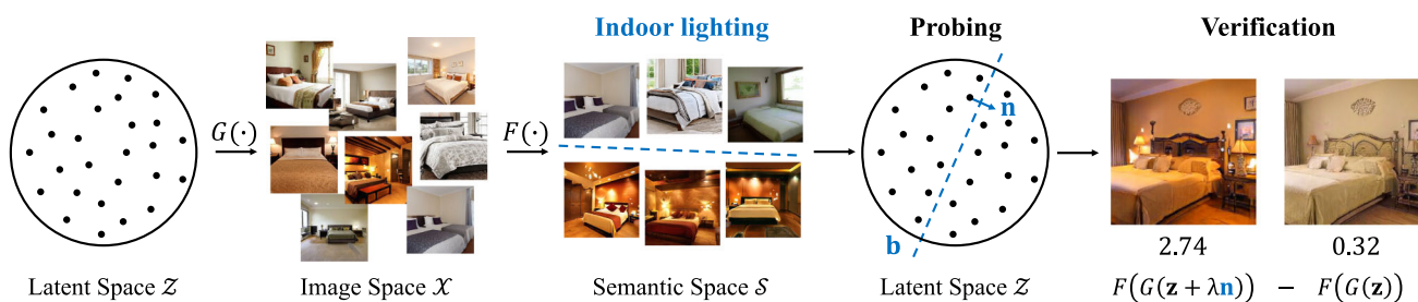
Fig. 4 Pipeline of identifying the emergent variation factors in generative representation. By deploying a broad set of off-the-shelf image classifiers as scoring functions, F(\cdot) , we are able to assign a synthesized image with semantic scores corresponding to each candidate variation factor. For a particular concept, we learn a decision boundary in the
