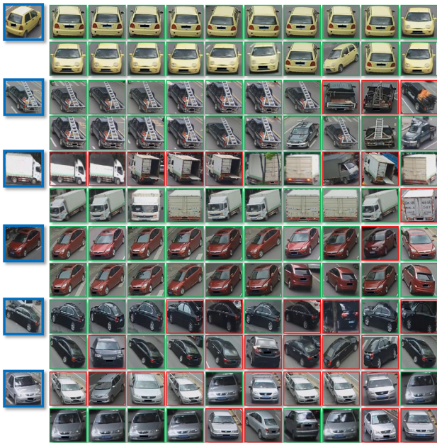
Fig. 12 Sample vehicle ReID results on VeRi-776. For each example, top-10 returned results of baseline and our VSCR are shown in the first and second row, respectively. Blue boxes are query vehicles. Red and green boxes denote false positives and true positives, respectively (Color figure online)
