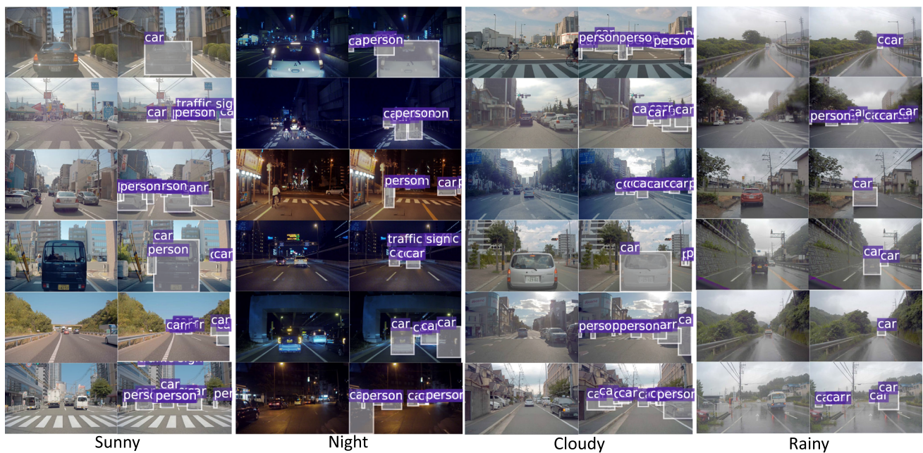
Fig. 4 Image samples from our benchmark grouped by their domain categories (sunny, night, cloudy and rainy). In each group, left are original images and right are images with corresponding bounding box annotations
