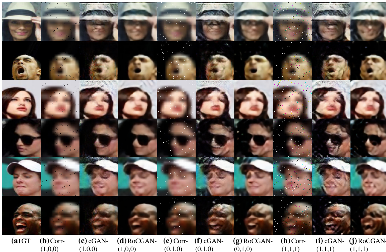
Fig. 4 Visual results depicting Bernoulli noise. Similarly to Fig. 10 different samples are visualized per row. The corrupted images are visualized in the original size to make the additional noise more visible. The
