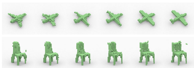
Fig. 7 Shape interpolation by linearly interpolating the encodings of the starting shape and ending shape
