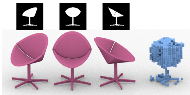
Fig. 11 Our method is unable to capture the concave interior structures in this chair shape. The pink shapes show the original shape used to generate the projected training data, shown by the three binary images on the top (in high resolution). The blue voxel representation is the inferred shape by our model. Notice the lack of internal structure
