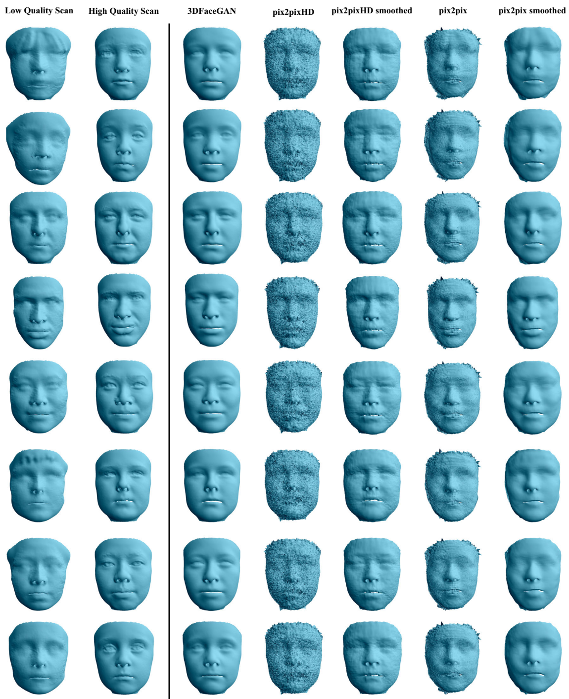
Fig. 9 The qualitative results of our approach compared to state-of-the-art baseline GAN methods in the 3D face translation task. The first column depicts the low quality input mesh whereas the second column represent the high quality ground truth meshes. We depict the raw results
