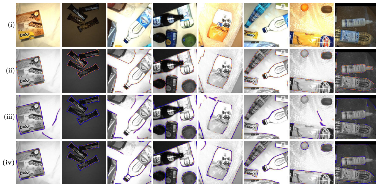
(a) Comparative results for instance boundary (blue) and occluding boundary side (orange) detection on D2SA. From top to bottom: input (i), ground truth (ii), prediction using the proposed network trained on D2SA (iii), using the proposed network pretrained on Mikado then finetuned on D2SA with the first three encoder blocks frozen (iv). Pretraining the proposed network on Mikado before finetuning on D2SA leads to significant improvements.
