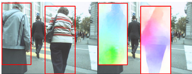
Fig. 7 We use the DPM (Felzenszwalb et al. 2010) person detector to crop out people from real-world scenes (left) and use SPyNet + SHOF to compute optical flow on the cropped section (right)
