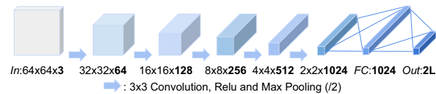
Fig. 2 Our plain CNN-6 network consisting of 5 convolutional and 1 fully connected layers followed by an output layer
