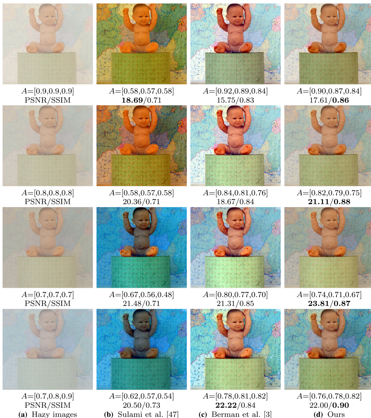
Fig. 6 Atmospheric light estimation on synthetic images. The method (Sulami et al. 2014) tends to under-estimate atmospheric light and results in darker dehazed results, while the approach by Berman et al.
