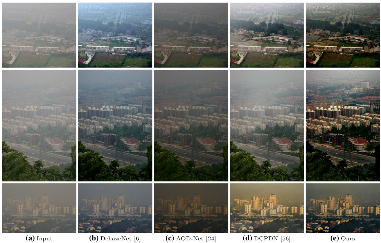
Fig. 14 Comparison on real-world thick hazy images with deep learning based methods. The methods of DehazeNet and AOD-Net tend to generate dark results, while the dehazed results by DCPDN have some non-uniform dehazing artifacts. In contrast, our results are more pleasant and have vivid scene details
