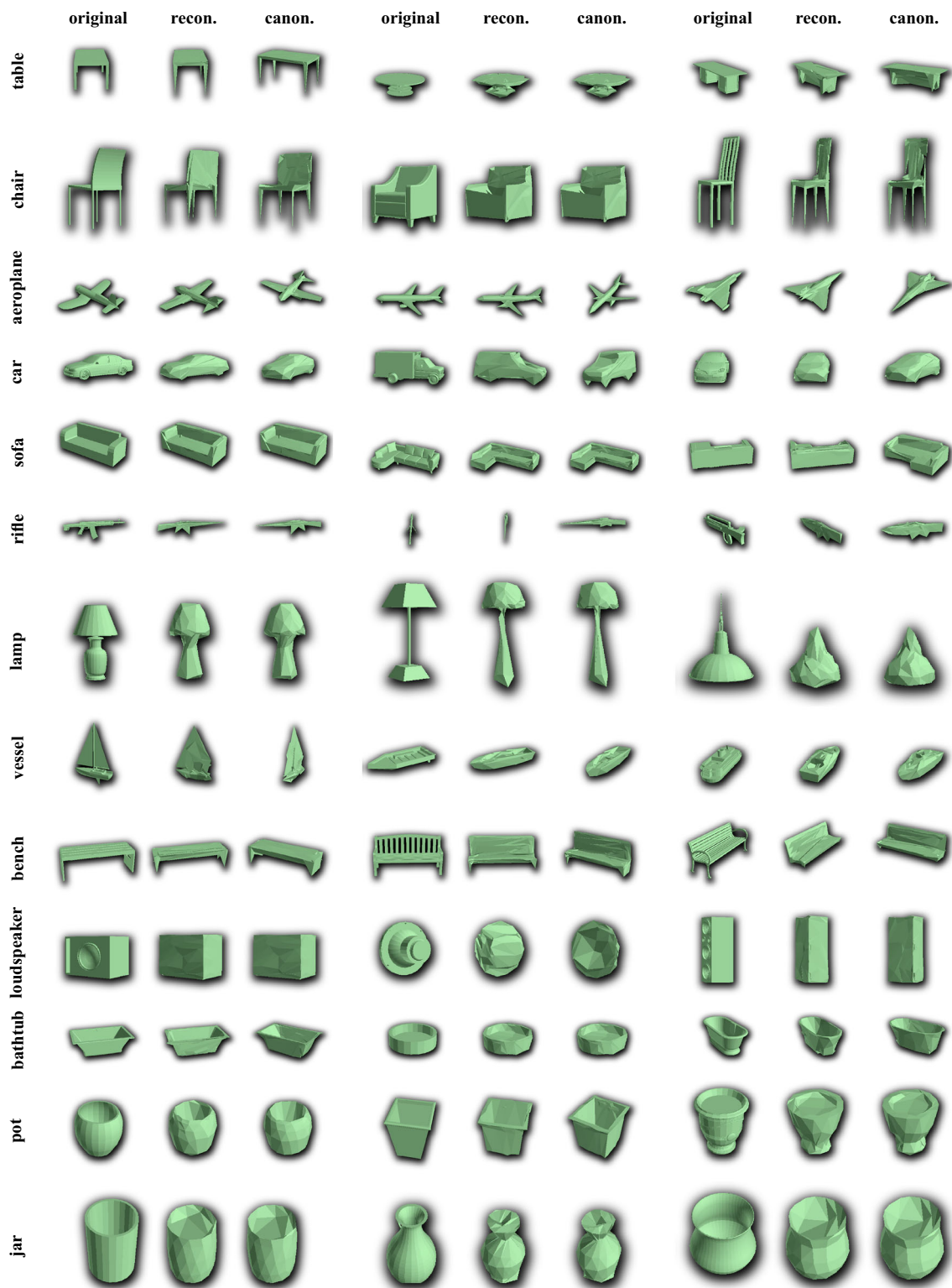
Fig. 6 Qualitative examples of reconstructions for different object classes. Each group of three images shows (i) ShapeNet ground-truth; (ii) our reconstruction; (iii) reconstruction placed in a canonical pose,
