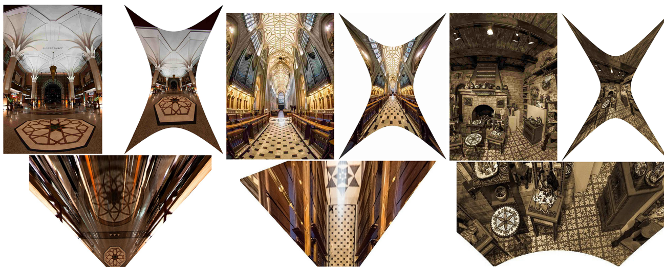
Fig. 3 Wide-angle results. Input (top left) is an image of a scene plane. Outputs include the undistorted image (top right) and rectified scene planes (bottom row). The method is automatic
