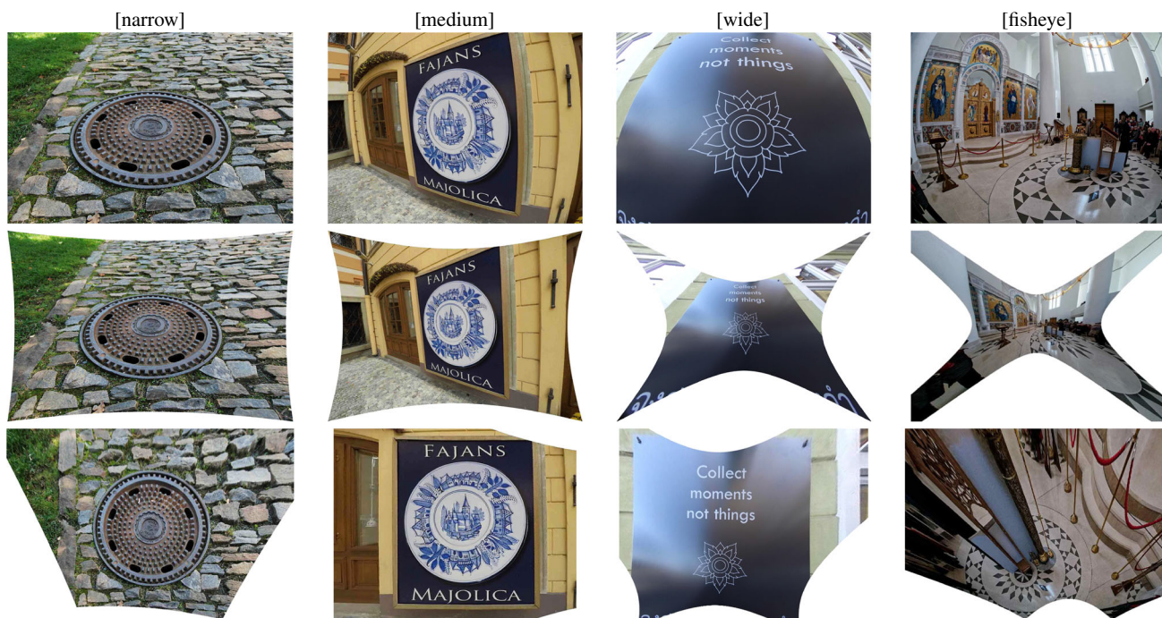
Fig. 11 Field-of-view study. The proposed solver H_{222}^{DES} \lambda gives accurate rectifications across all fields-of-view: (left-to-right) Nikon D60, GoPro Hero 4 at the medium- and wide-FOV settings, and a Panasonic
