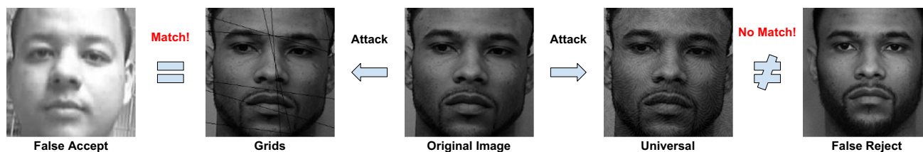
Fig. 1 Illustrating how an image can be attacked with perceptible and quasi-imperceptible adversarial perturbations to create false accepts (match between different individuals) and false rejects (non-match
