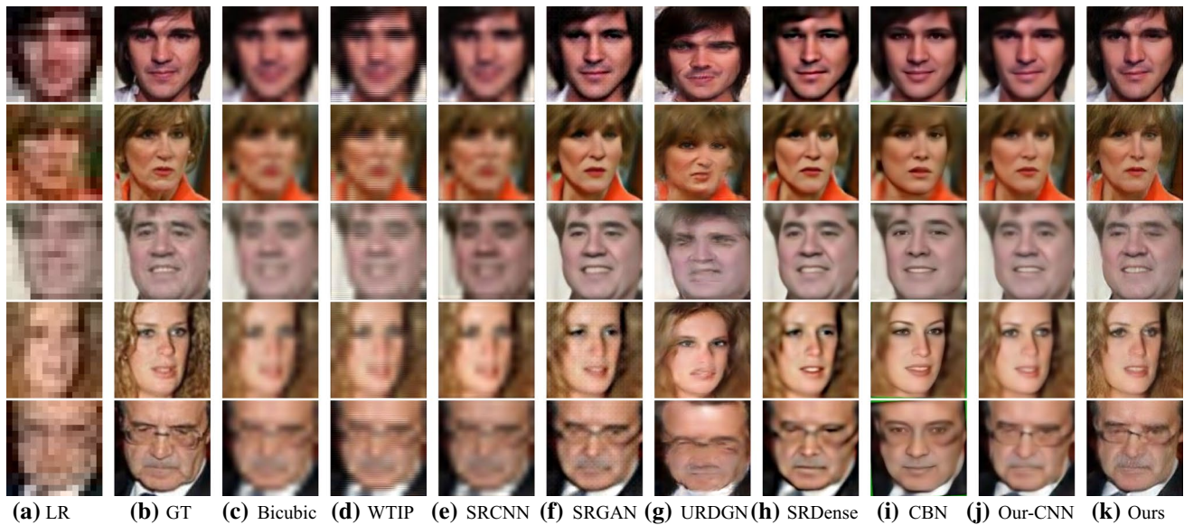
Fig. 8 Comparison with the state-of-the-art methods on 16 \times 16 input resolution with 8\times upscaling factor. All the images are randomly selected from the LFW dataset
