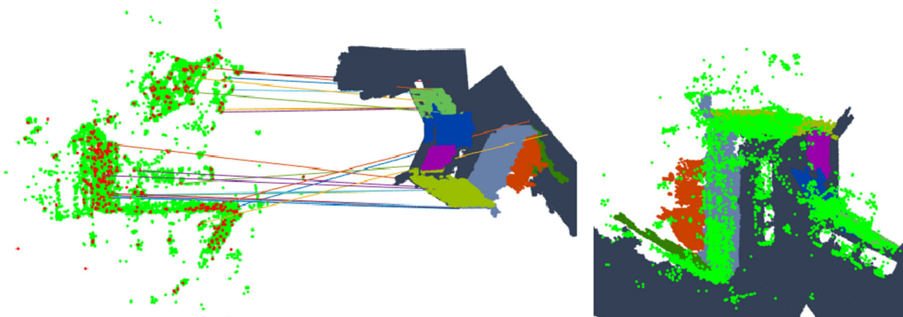
Fig. 9 Point-to-plane registration for Scene73 with correspondences. Left: recovered point-to-plane correspondences with all the processed points in red. Right: registration between reconstruction (in green) and the segmented scene (Color figure online)
