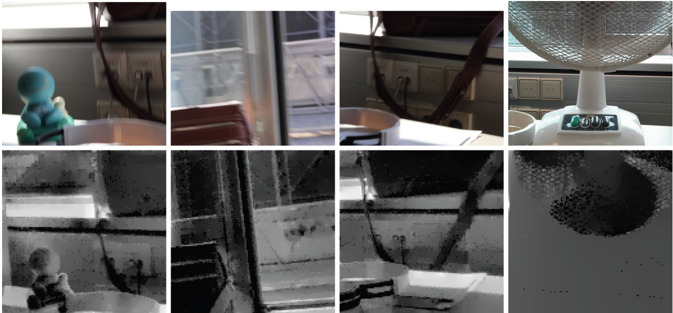
Fig. 8 Comparison to a video captured with a modern DSLR camera. Notice the rather strong motion blur in the images of the DSLR (top row), whereas the DVS camera can easily deal with fast camera or
