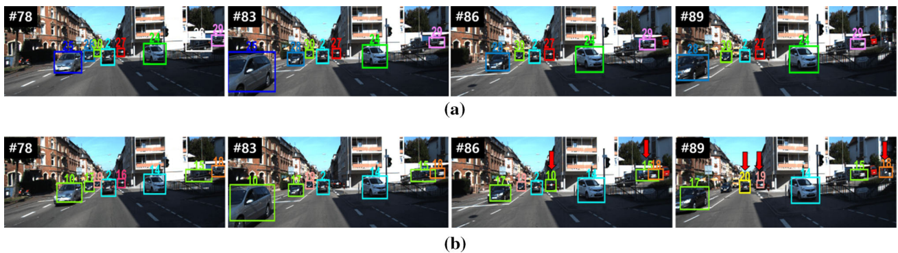
Fig. 13 Qualitative comparisons on the KITTI0011 sequence. a SCEA. b RMOT (or RMN-HM): the label of object 16 at #78 is changed at #86 (16→10). The labels of object 2 and 10 at #86 are changed at #89 (2→20, 10→19). The label of object 18 at #86 is incorrectly assigned to a new object at #89
