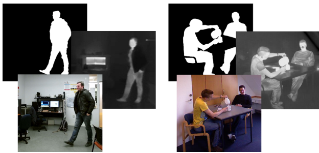
Fig. 1 Examples of mutual foreground segmentation in low contrast conditions for RGB-LWIR image pairs. On the left, the person is only partly perceptible in the LWIR spectrum due to a winter coat, but is clearly perceptible in the visible spectrum. The opposite is true on the right, where legs are hard to perceive in the visible spectrum, but easy to perceive in the LWIR spectrum
