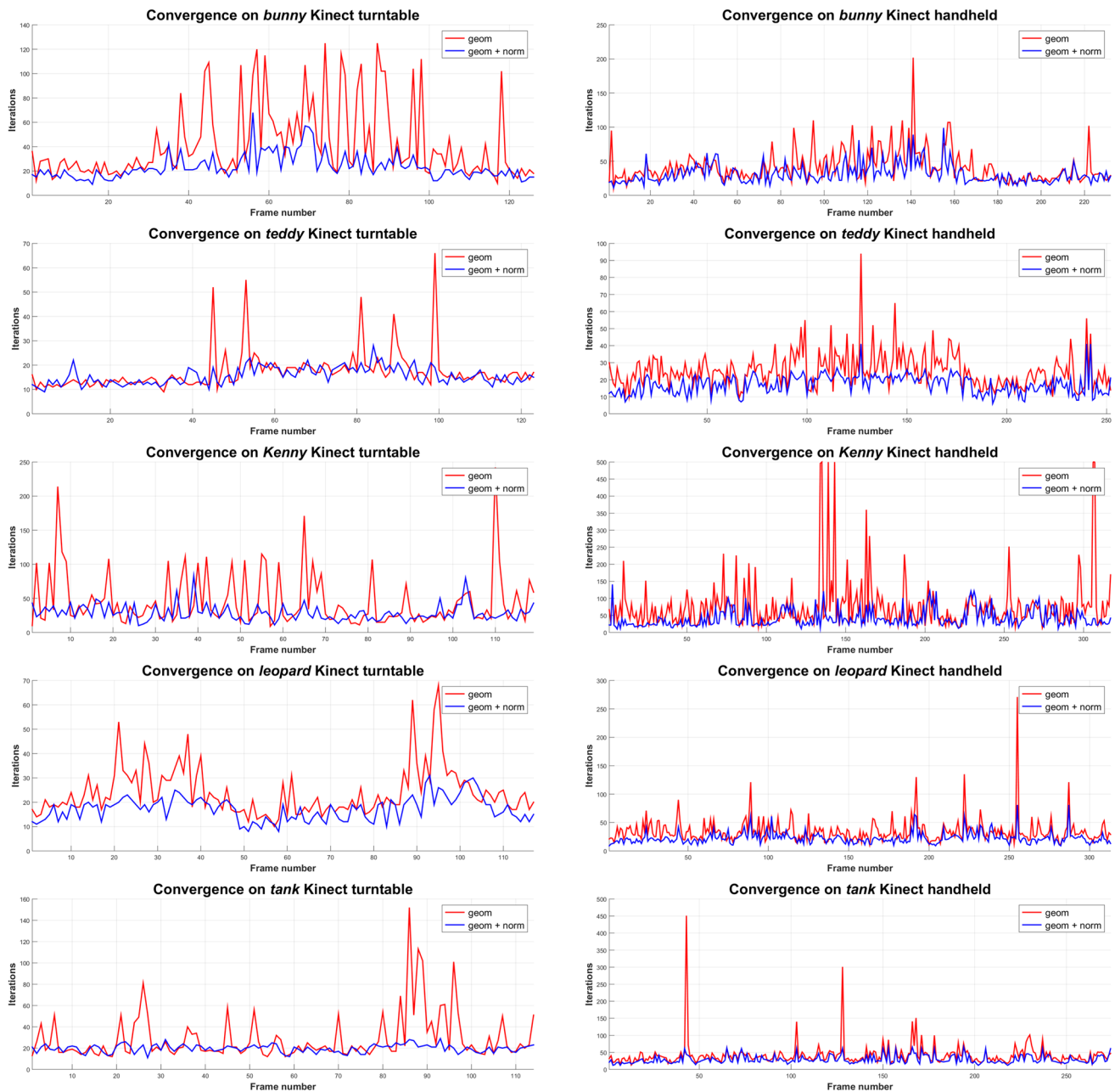
Fig. 10 Comparisons of iterations to convergence with E_{geom} versus E_{geom} + E_{norm} on Kinect sequences
