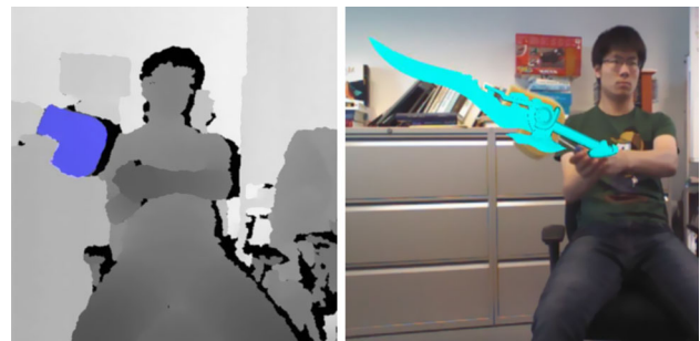
Fig. 1 Illustration of our method tracking an arbitrary object and enabling its use as a game controller. On the left we show the depth image overlaid with the tracking result and on the right we visualise a virtual sword with the corresponding 3D pose overlaid on the RGB image
