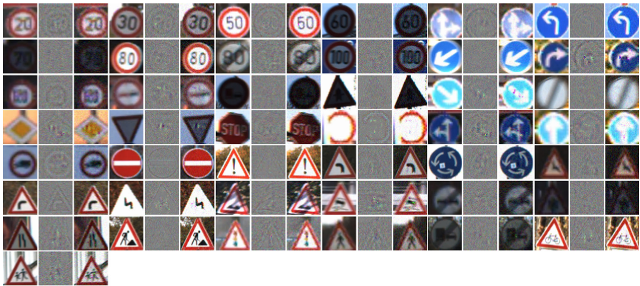
Fig. 9 Minimum additive noise which causes the traffic sign to be misclassified by the minimum different compared with the highest score (best viewed in color and electronically) (Color figure online)
