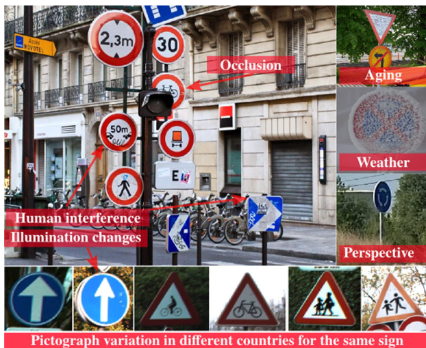
Fig. 1 Some of the challenges in classification of traffic signs. The signs have been collected in Germany and Belgium
