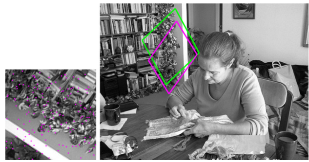
Fig. 4 Example from a Fast-Match Run. Left The template (shown enlarged for clarity), with the 152 pixels that Fast-Match samples. Right Target image, with origin of the template (ground truth location) in green and a candidate area it is mapped to in magenta
