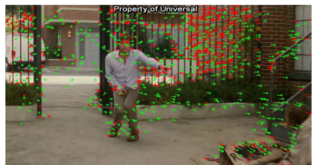
Fig. 2 Visualization of inlier matches of the estimated homography. Green arrows correspond to SURF descriptor matches, and red ones are from dense optical flow (Color figure online)
