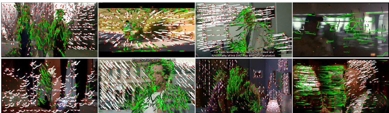
Fig. 3 Examples of removed trajectories under various camera motions, eg, pan, zoom, tilt. White trajectories are considered due to camera motion. The red dots are the feature point positions in the cur-
