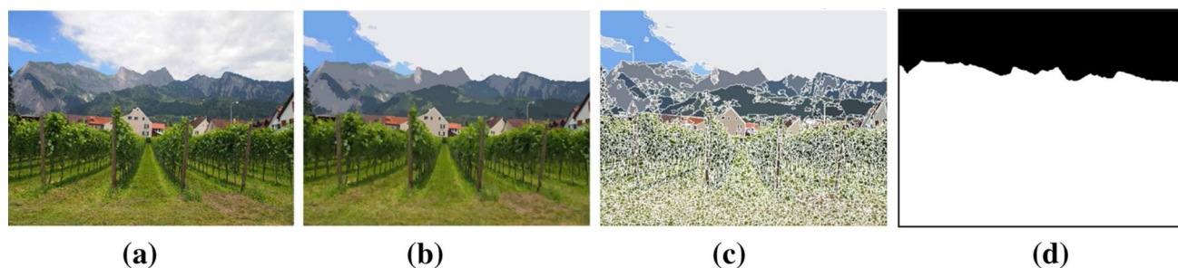
Fig. 2 Superpixel based segmentation: a Input image. b MeanShift filtered image. c MeanShift region boundaries. d Final segmentation
