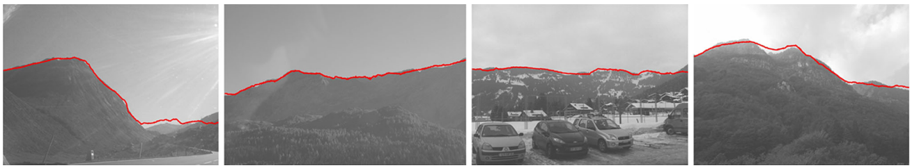
Fig. 9 Some incorrectly localized images. This usually happens to images with a relatively smooth skyline and only few distinctive features. The pipeline finds a contour that fits somewhat well, even if the location is completely off
