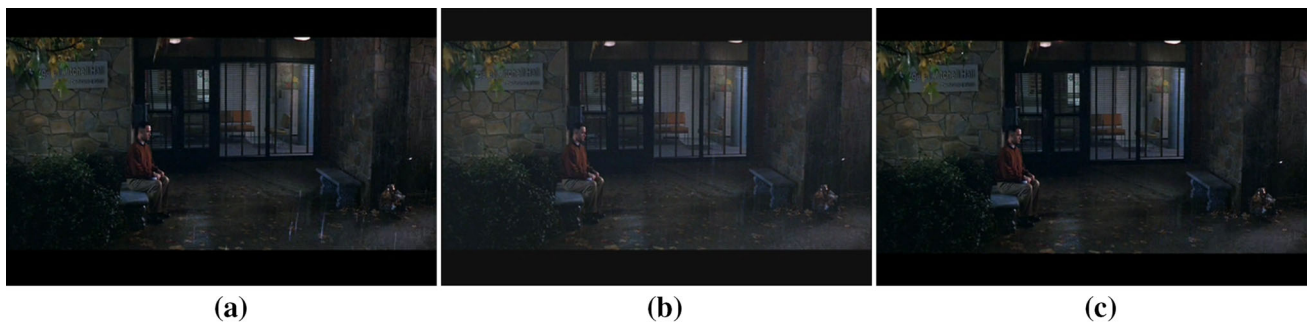
Fig. 15 Qualitative comparison for video with global motion. a Original frame with rain, b frame with rain removed by Barnum et al. (2010), c frame with rain removed using proposed technique
