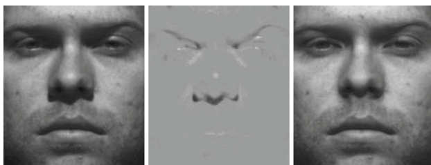
Fig. 6 Removal of non Lambertian effects. On the left we show one of the input images. In the middle image we show the detected non Lambertian components (shadows and specularities) via the low-rank matrix recovery pre-processing step. Finally, on the right image we show the low-rank and noise-free data used in our algorithm
