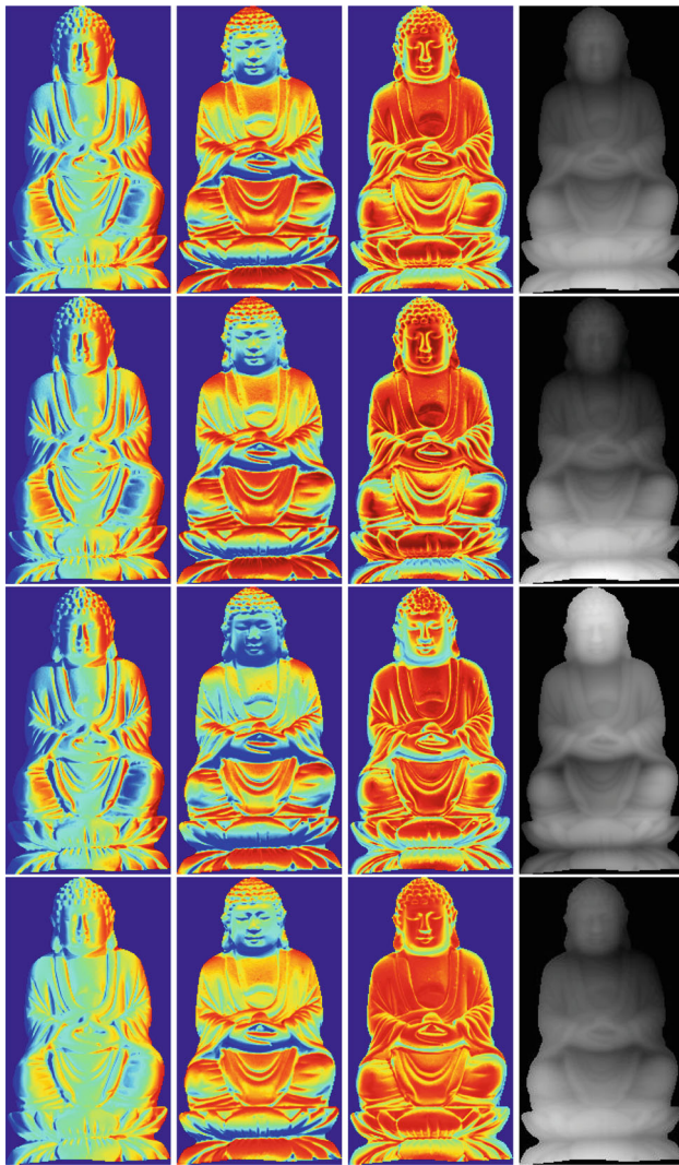
Fig. 7 Comparison of reconstructed normal and depth maps. From left to right, each column corresponds to the first ( x axis), second ( y axis), and third ( z axis) components of the normal map \mathbf{n} and the depth map, respectively. We show the results obtained from the calibrated photometric stereo method (top row), the results obtained from our method (second row), the results obtained from the entropy minimization method (third row) and the results obtained from the SCPS method (bottom row)
