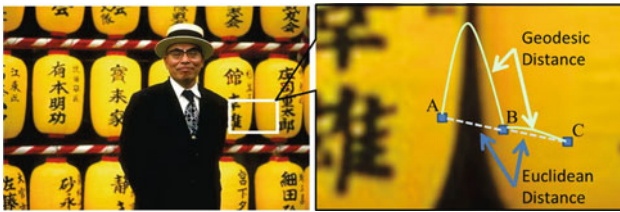
Fig. 2 Geodesic distance versus Euclidean distance: Image contents in-between could provide a crucial evidence for measuring the similarity between two pixels
