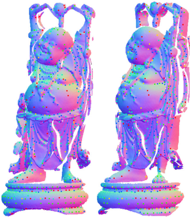
Fig. 3 Scale-dependent corners computed based on geometric scale-space analysis of two range images. The range images are depicted with their normal fields. The scale-dependent corners are colored according to their inherent scales. Red, yellow, green, turquoise and blue dots indicate the corners detected from the coarsest to the finest scales (Color figure online)
