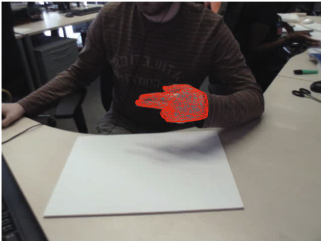
Fig. 5 The average processing time when using the model on top with the image on the bottom is 2.91 ms. The resolution of the images is 640 \times 480 and the model has 680 triangles
