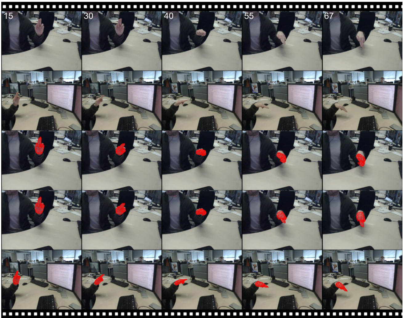
Fig. 18 Multi view tracking. The top two rows show the two views. When processing only the first view ( top row ) the results are incorrect ( third row ) because the silhouette to pose mapping is ambiguous (mul-
