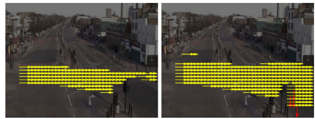
Fig. 9 Example of fine grained cluster decomposition discovered: strictly horizontal vs. turning flows
