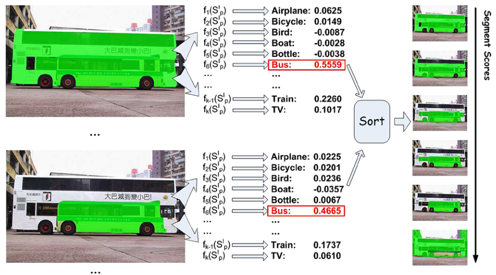
Fig. 4 An illustration of our segment categorization process. Each segment is given as input to regressors specialized for each category, producing estimated qualities. The maximal score across categories is used to sort segments and decide on their category
