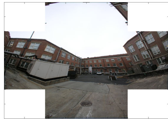
Fig. 11 Cubemap of undistorted left image (unwarping done using a simple line interpolation between \theta and r , the distorted radius)
