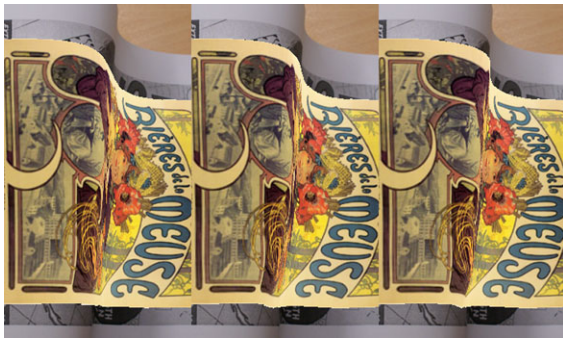
Fig. 15 Close-up view of Fig. 14g (left) where only keypoints were used for registration, Fig. 14m (middle) where pixel-based registration was used including over-smoothing penalty to self-occlusions and Fig. 14s where a shrinker term is used in self-occlusions
