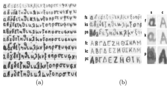
Fig. 11 Test images. (a) The same ink was used to write ten layers of the Greek alphabet at ten different densities. (b) Test images capture the writing behavior of an author as it is influenced by pen type and letter size. Penna type (p) often results in accidental ink spills and larger spread areas, as opposed to the terser kalamus (k) and feather (f)
