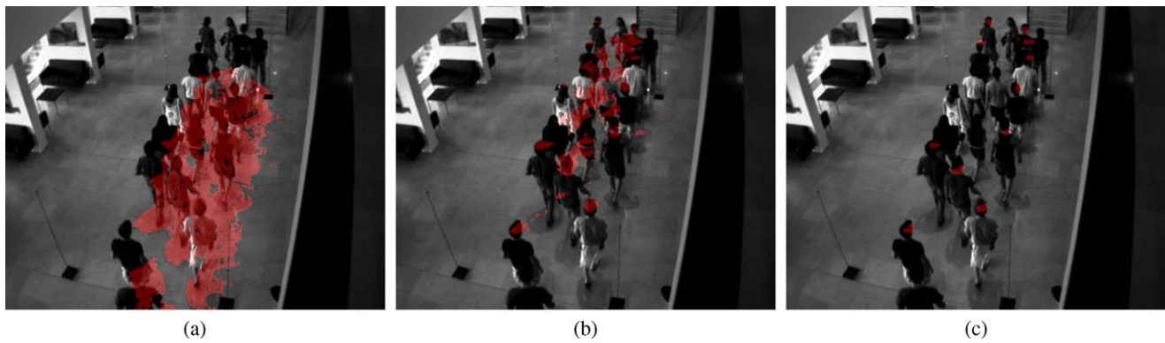
Fig. 3 Intensity correlation improves detection. (a) Combined foreground from all views, without using intensity correlation, at ground plane. Detection result is a single large blob, containing most of the people in the scene. (b) Same as (a), but for height 170 cm. Detection results at the head height are significantly improved compared to those at the ground plane, but still the number of false positives, specifically
