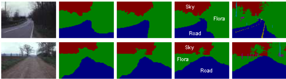
Fig. 11 Qualitative object segmentation and recognition results. The first column shows the original image from the Sowerby-7 dataset. Column 2 shows the result of performing inference in the pairwise CRF model described in Sect. 2. The result obtained using the P^n Potts
