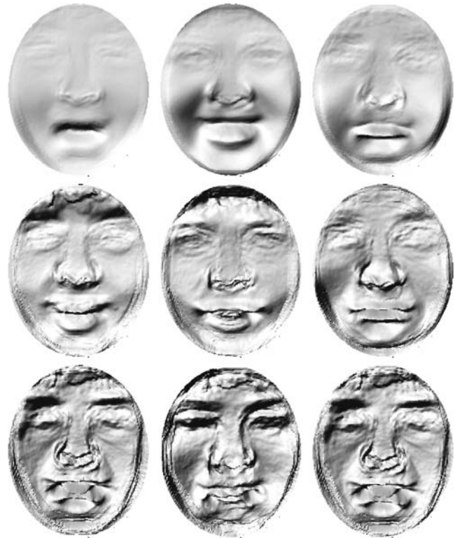
Fig. 3 Some eigenvectors which span the shape residue PCA subspace (our expression deformation model). The images in the top row are the 1st, 2nd and 3rd eigenvectors, respectively from the left. The 9th, 10th and 11th are in the middle row and the 25th, 26th and 27th are in the bottom row. Notice that the top eigenvectors are more relevant to the largely deformable regions (e.g. the mouth) and the deformations in the other regions gradually appear in the lower eigenvectors
