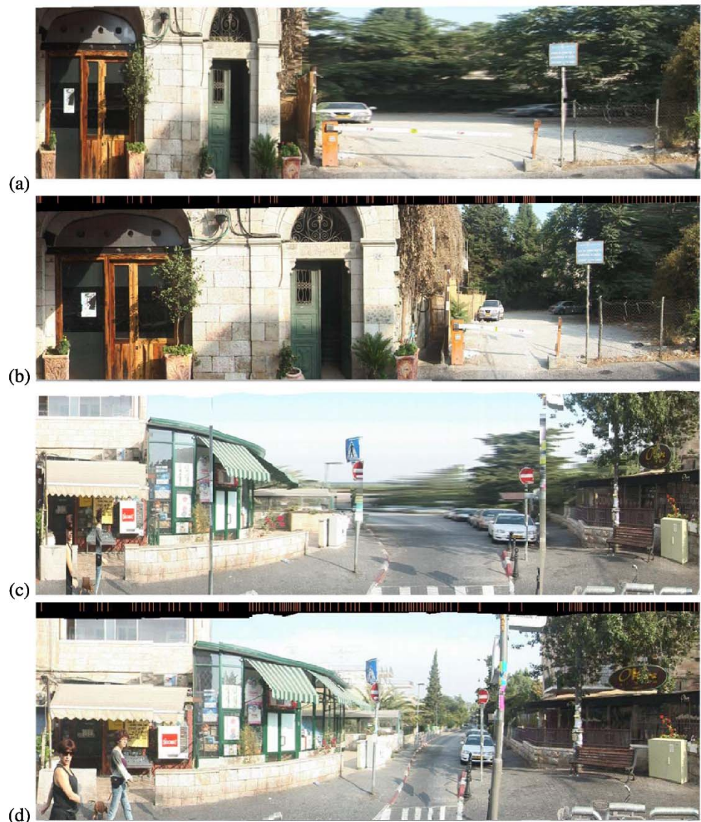
Fig. 11 Pictures (a, c) are segments from a long pushbroom mosaic, while (b, d) show the same area in a long MAD mosaic. Substantial widening of far away objects and narrowing of close objects is evident in pushbroom. While width of strips is uniform in pushbroom, strip boundaries are marked on top of the MAD Mosaic image. Note also that the MAD mosaic avoids cutting inside moving objects
