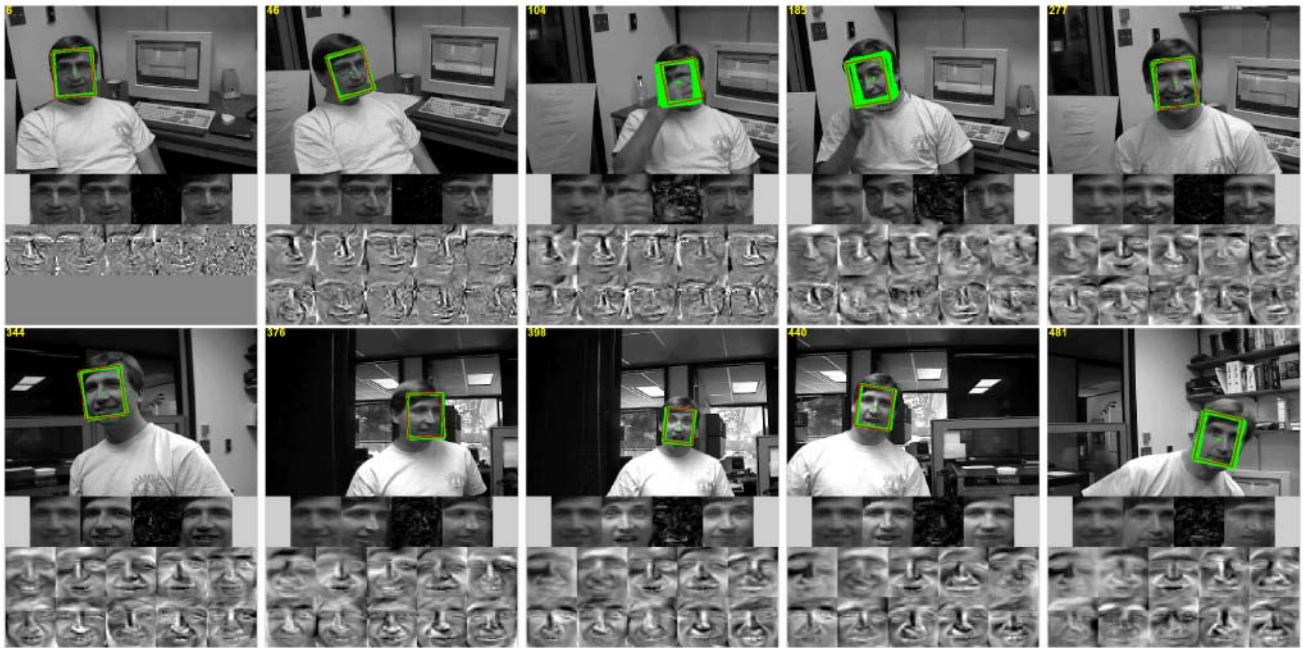
Fig. 4 (Colour online) A person undergoing large pose, expression, appearance, and lighting change, as well as partial occlusions. The red window shows the maximum a posteriori estimate of the particle filter, and the green windows show the other particles with weight above a threshold. The results can be better viewed on high resolution displays or color printouts. More results are shown in the accompanying video
