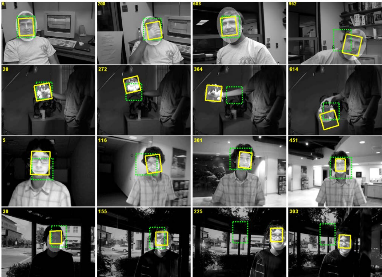
Fig. 10 (Colour online) A comparison of our tracker (indicated with a yellow box) with the WSL (Jepson et al. 2003) (shown in highlighted ellipse) and the Mean Shift (Comaniciu et al. 2003) (depicted by a green dashed box) on four video sequences
